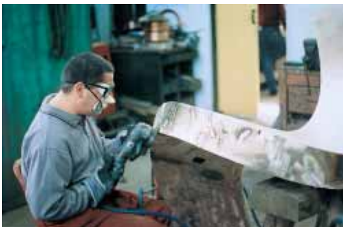
The worker is exposed to noise during grinding. He should be wearing ear defenders
